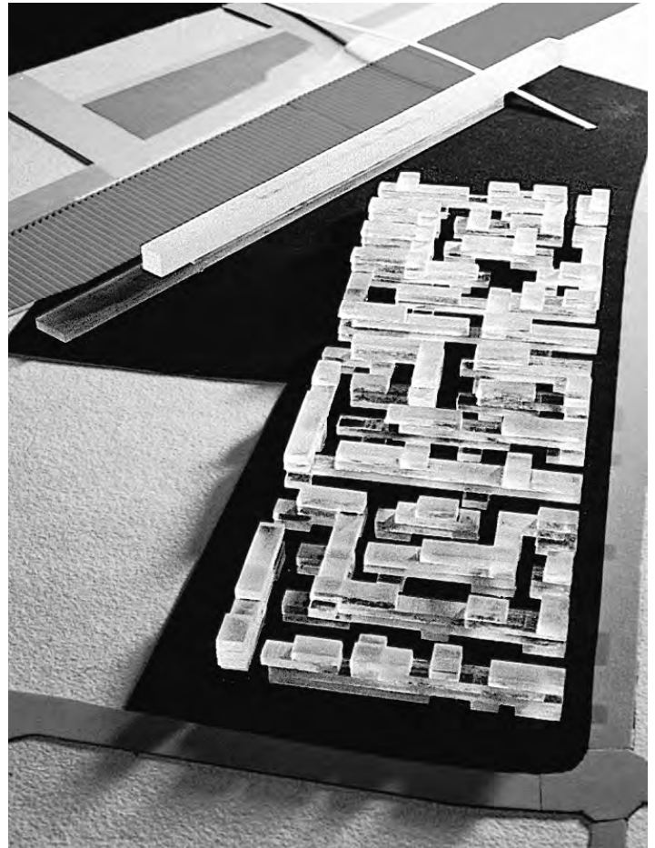
Two and partially three story carpet housing consisting of various sizes of modular units which benefit from an optimal exposure to day-light and roof terraces
