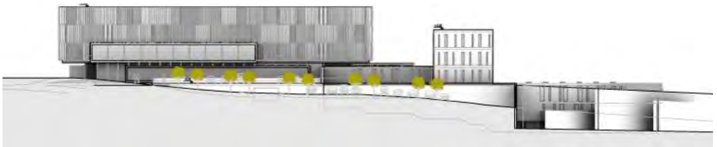
Longitudinal section showing the basement level as a plinth of the light structure
