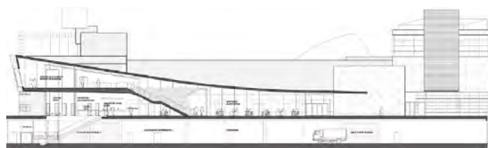
Longitudinal section through the pavilion showing the connection to the garage
